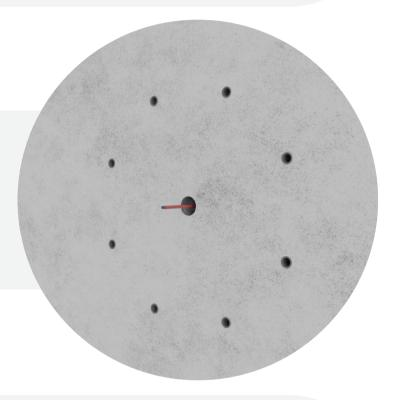
If utilizing the provided **Cement Plugs**, drill holes measuring 8mm in diameter. Insert the plugs securely into each hole.
